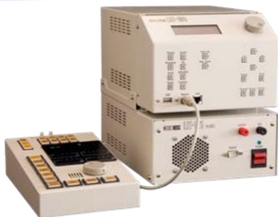
LVDS Inspection System for TV LIT-101
